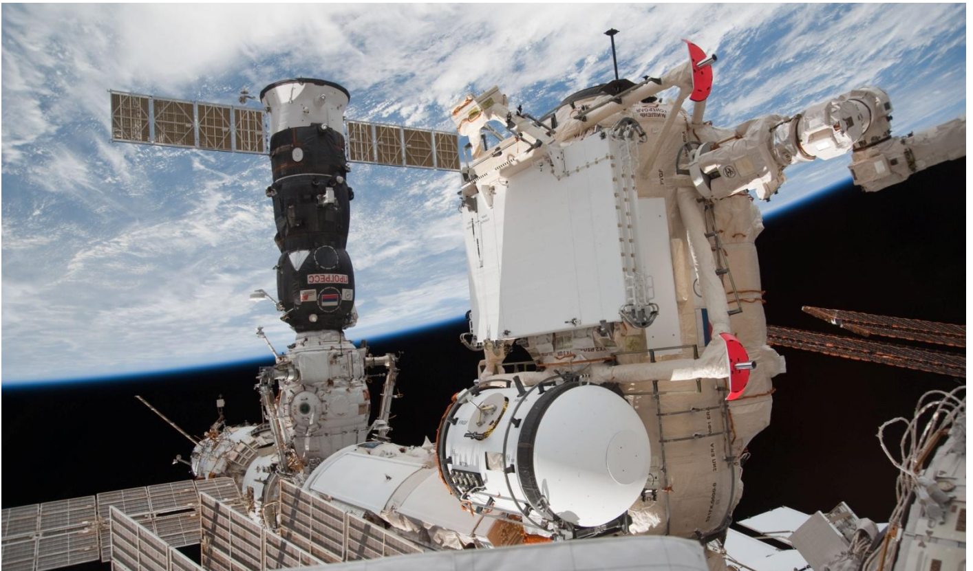
(Above) Atlantis docked to the ISS, with the Russian-built Rassvet module visible in its payload bay. (Below) In the grasp of the station's robot arm, Rassvet is attached to the Earth-facing port of the Zarya module of the International Space Station. (NASA)
