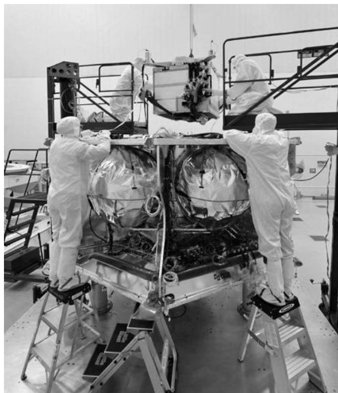
Workers place the special radiation vault for NASA's Juno spacecraft onto the propulsion module. Juno's radiation vault has titanium walls to protect the spacecraft's electronic brain and heart from Jupiter's harsh radiation environment. The whole vault, with more than 20 electronic assemblies inside, weighs about 200 kilograms. This image was taken on 19 May 2010, in the high-bay cleanroom at Lockheed Martin Space Systems in Denver, during Juno's assembly process. (NASA/JPL-Caltech/LMSS)
