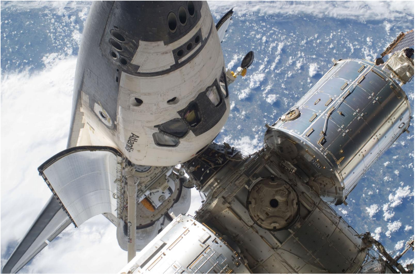
(Above) Atlantis docked to the ISS, with the Russian-built Rassvet module visible in its payload bay. (Below) In the grasp of the station's robot arm, Rassvet is attached to the Earth-facing port of the Zarya module of the International Space Station. (NASA)
